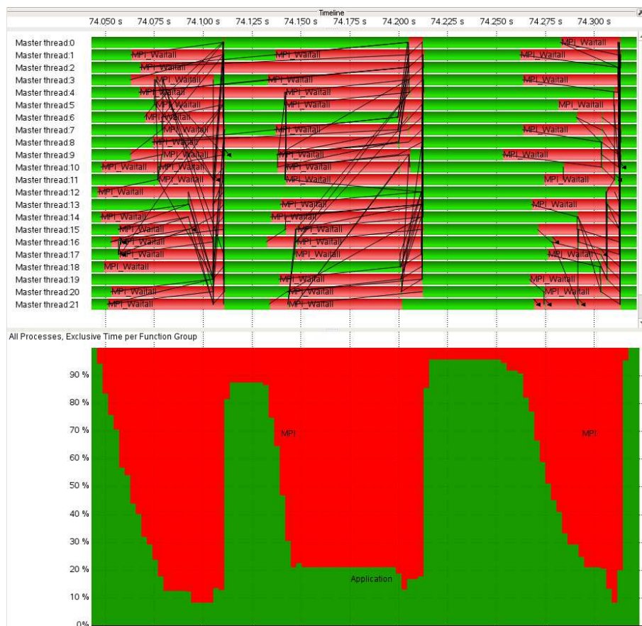
Figure 15: Application code load imbalance and its effect on MPI
